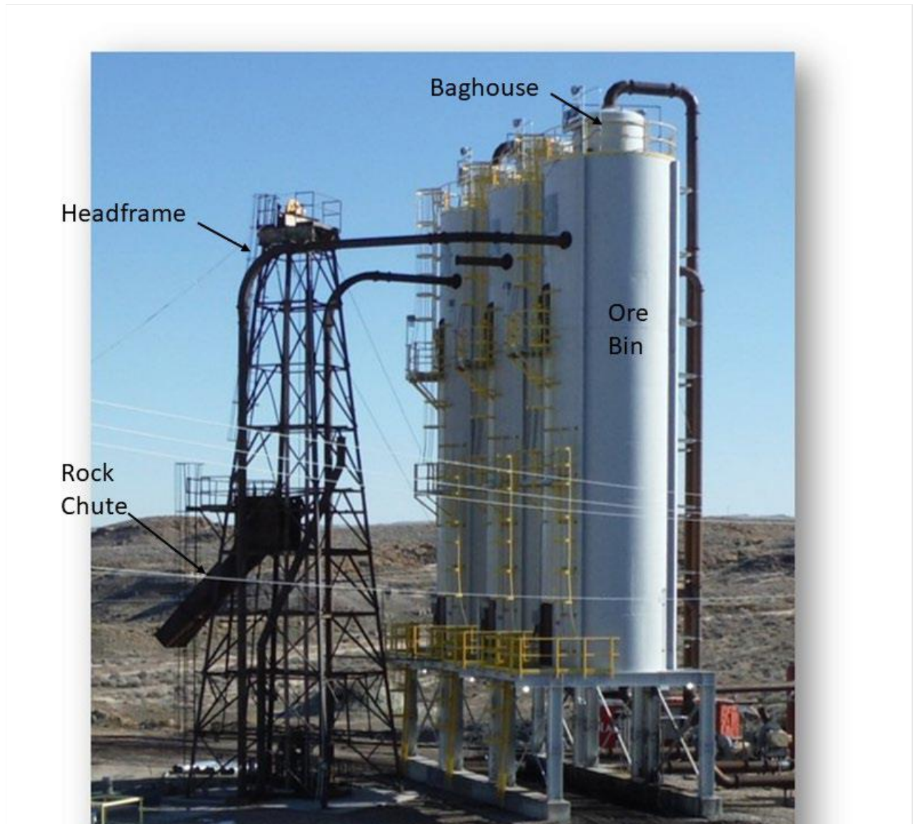
Figure 3. Photo of typical surface set up at a working gilsonite mine shaft
