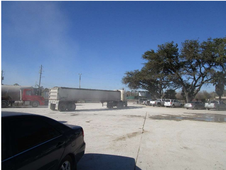
Dust emissions from aggregate transportation on dusty pavement
