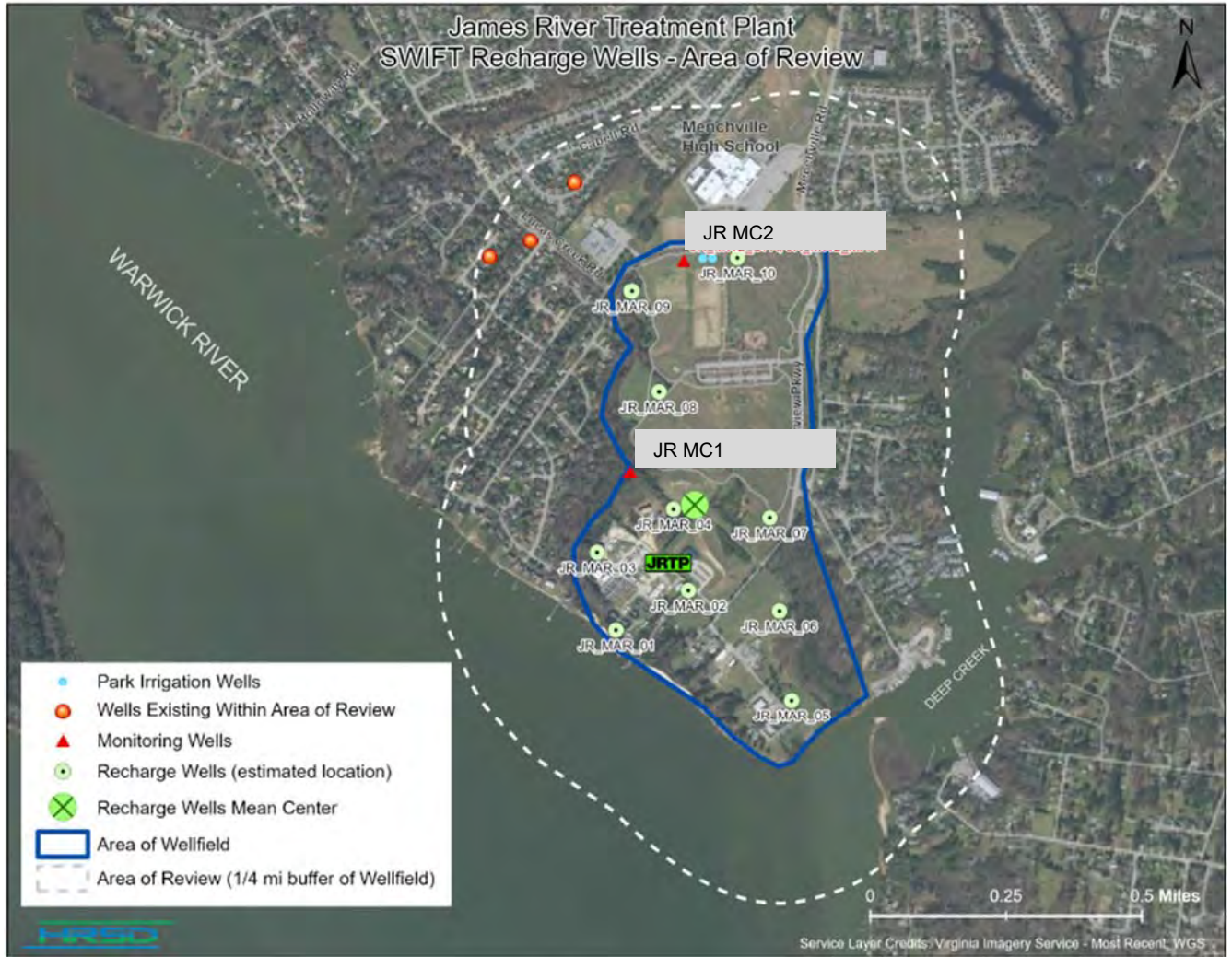
Figure 1.1: Proposed locations of Managed Aquifer Recharge (MAR) Wells for JR SWIFT and monitoring wells. MAR and monitoring well locations may be adjusted based on site specific conditions but will lie within the area of the wellfield denoted by the blue boundary. Private wells are identified in blue and red. The three private wells that have been constructed within the AOR are less than 50 feet deep and screen the surficial Columbia Aquifer. All existing and potential future wells based on available permit applications are classified as non-potable and each of these private well users is connected to the public water supply for potable water use (Newport News Waterworks). The brackish groundwater quality contained in the UPA and MPA makes using these aquifers for potable, irrigation, commercial, or industrial supplies impractical. Note well features are not to scale.
