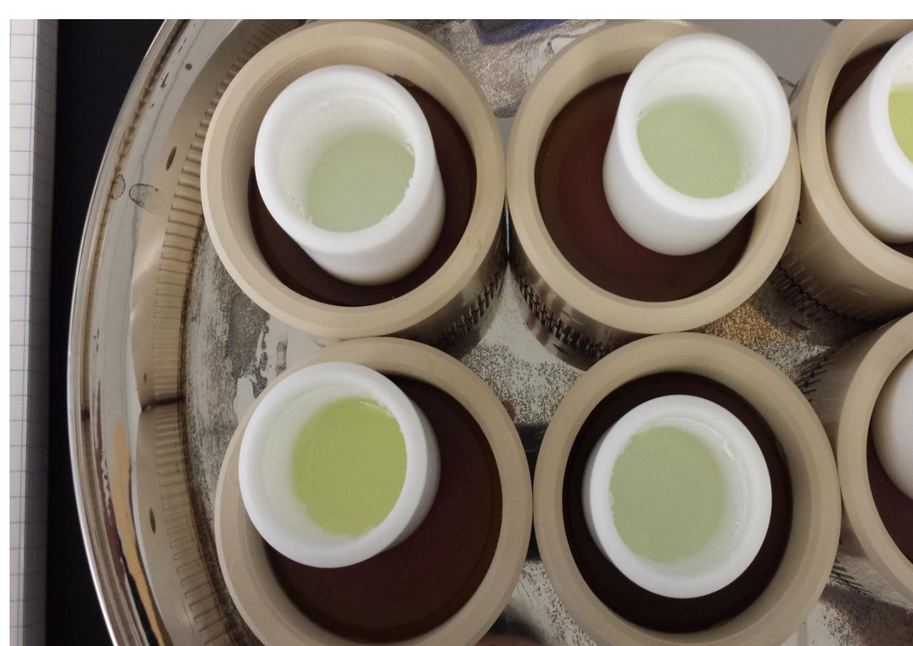
Figure 2. Moss samples after microwave assisted acid digestion in preparation for Hg quantification with Tekran 2600.
