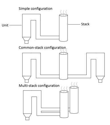
Figure 1: Unit-to-stack configurations
