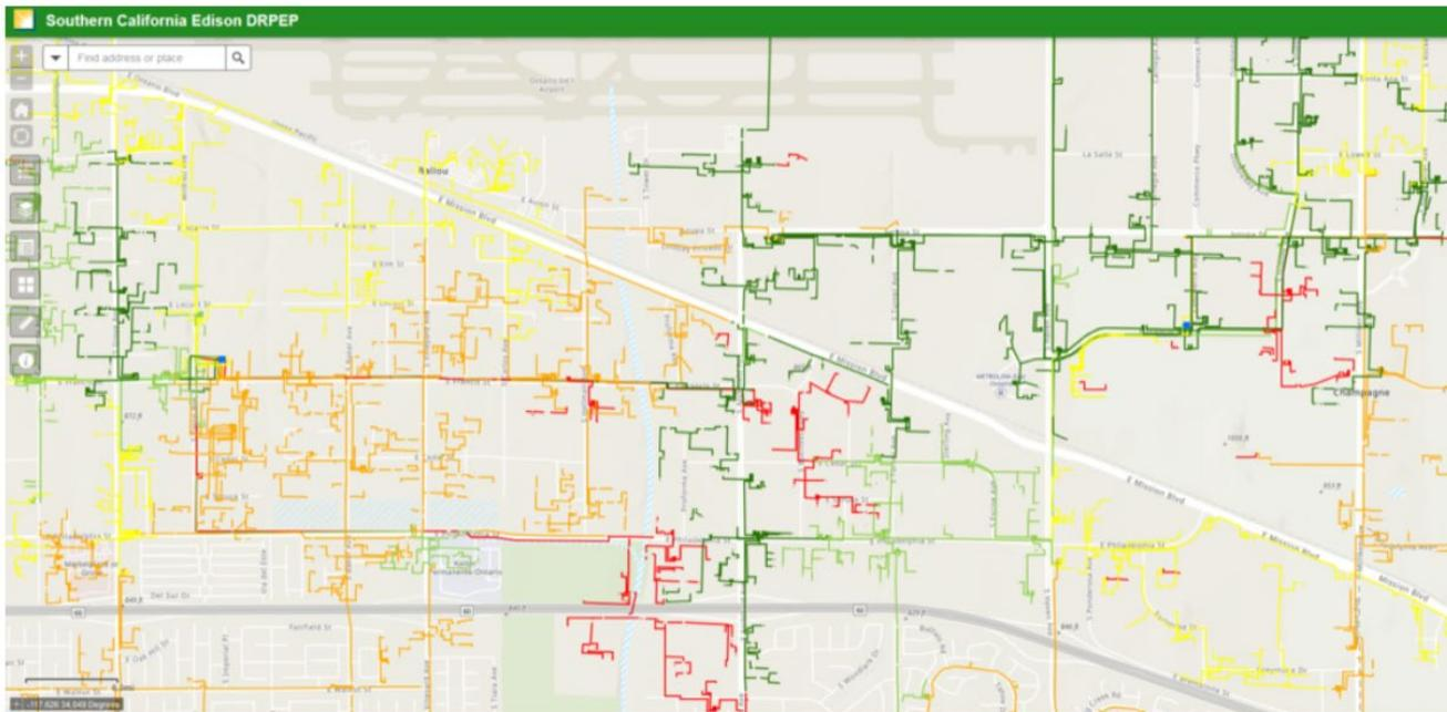
Source: (IREC 2019). Color scale indicates the available capacity on the line, with red indicating the most limited, orange, yellow, and light green each indicating higher levels of capacity, and dark green indicating ample capacity.
