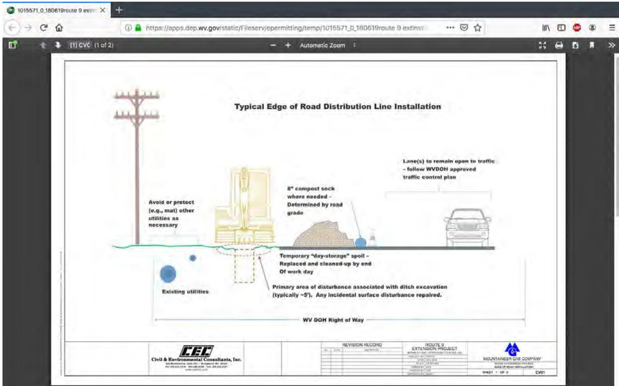
**EXHIBIT XX - CONSTRUCTION METHOD FOR EDGE OF ROAD (LONGITUDINAL)
