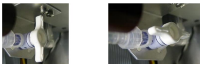
Purge valve closed (Left) and open (Right). Located inside the battery compartment
