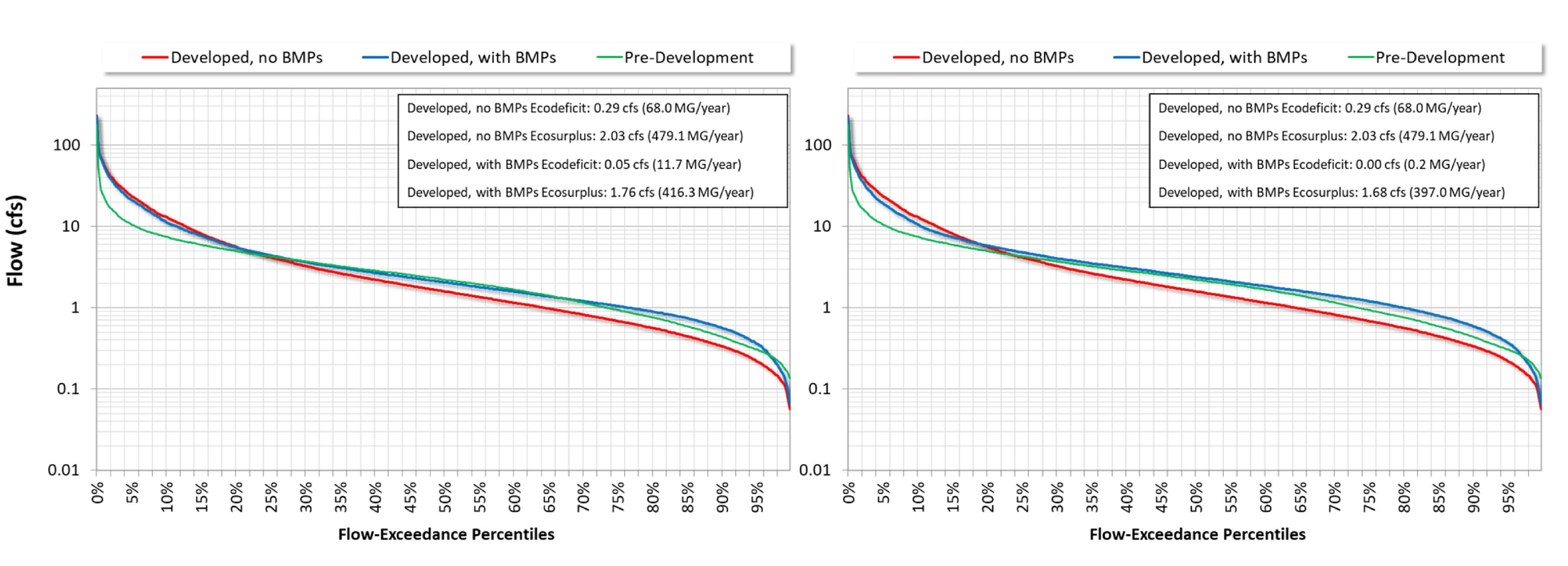
Flow duration curve with MS4 control SCMs treating 80% of the Upper Hodges Brook subwatershed's impervious cover under historic LULC and climate conditions
