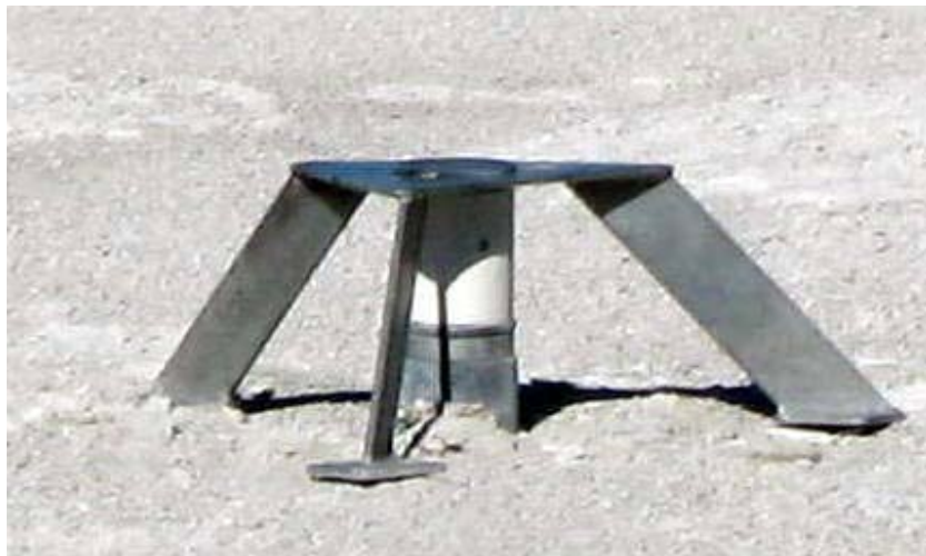
Figure 2.5 - A Height Adjustment Tool is used to measure the height of Sensits and CSCs and to adjust the sensor and inlet height to 15 cm above the soil surface.
