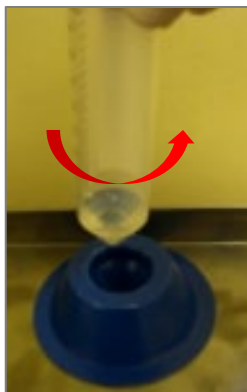
Gentle swirl of tube with carrier after addition of 4 mL disinfectant/control substance.
