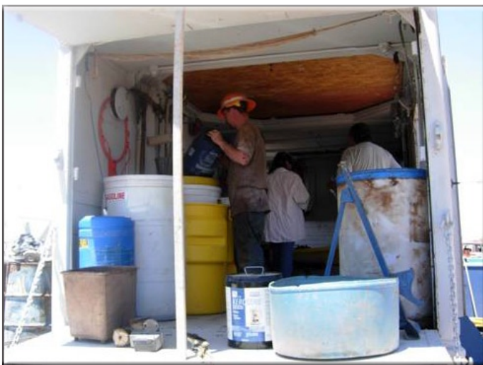
Fluid collection at the Hopi Tribe. The tribe subcontracts all activities to prepare the vehicles for crushing. Fluids are removed from the vehicle and placed into secondary containers. Anti-freeze and oil are recycled. Mercury switches are handled and disposed of as hazardous waste. Gasoline is disposed of by an environmental waste management service.
