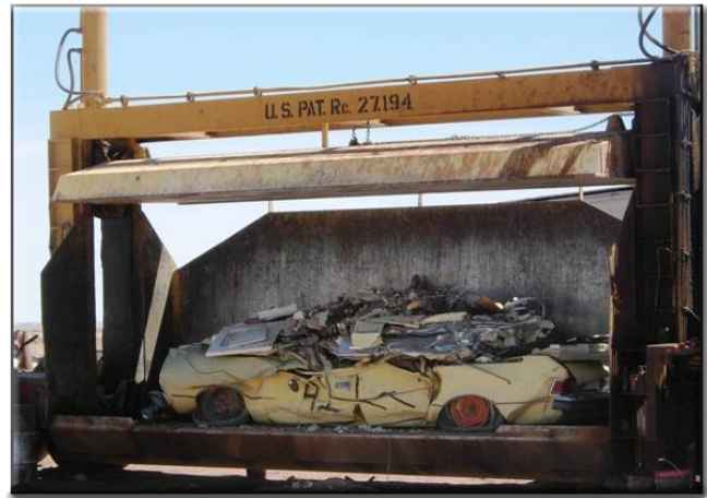
Vehicle crushing by the Hopi Tribe. The crusher is contracted by the Tribe and arrives to crush vehicles collected in a centralized location. To reduce cleanup needs crushing should take place over drip pads or other absorbent material.
