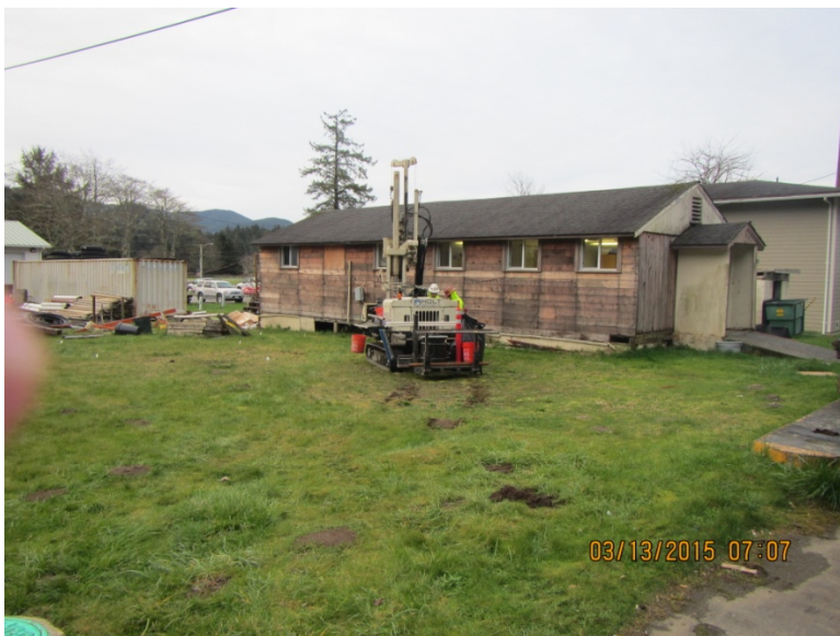
Photo 49. UST E Groundwater grab sampling (AQE1)
