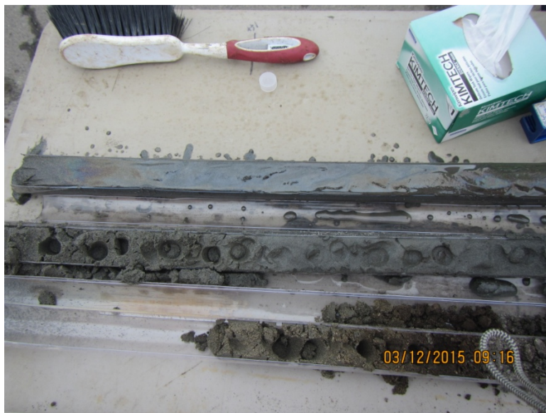
Photo 42. GP-11-CD18 0-15 ft bgs (top) with visible sheen through 10-15ft bgs interval
