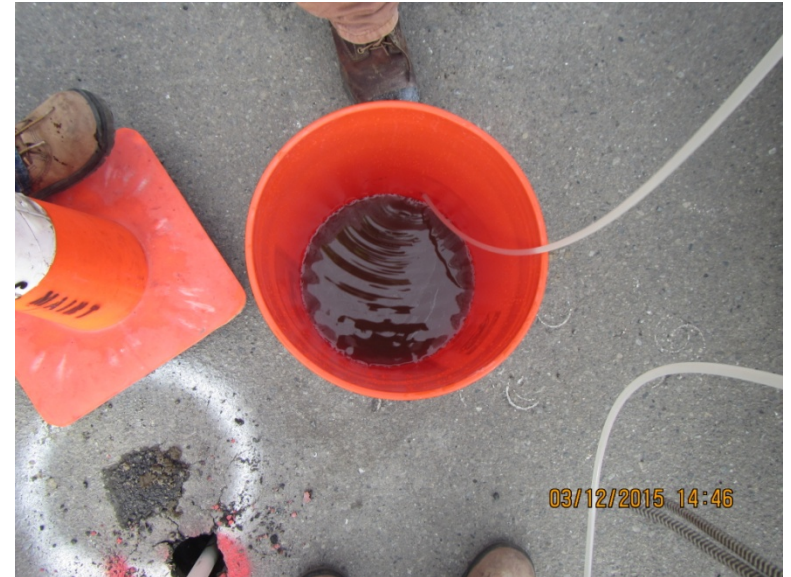
Photo 47. AQCD2 purge water with sheen
