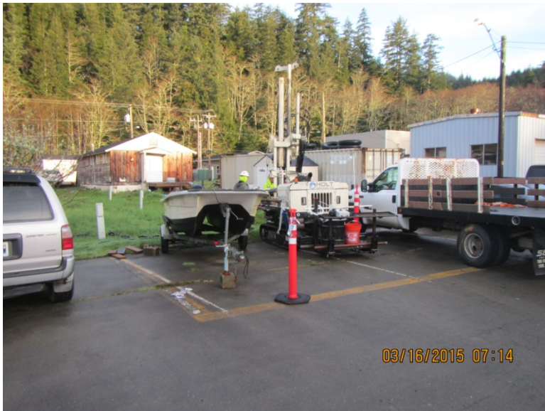
Photo 54. UST E Groundwater grab sampling (AQE3)
