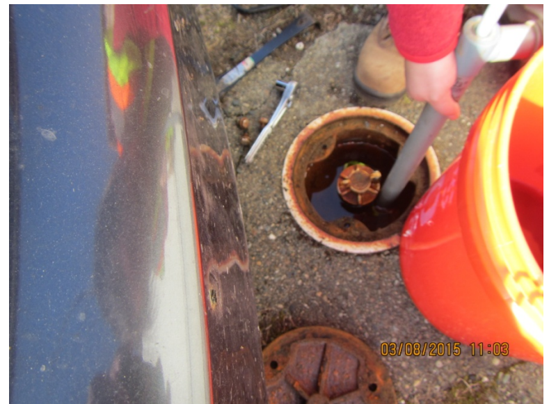
Photo 28. Purging water out of well casing at MW-5
