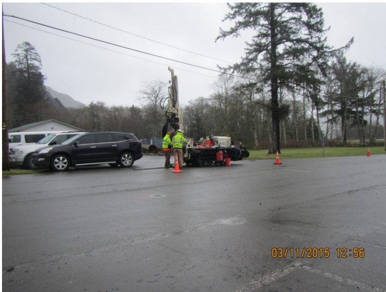
Photo 38. USTs C/D step-out sampling (GP-11-CD19)
