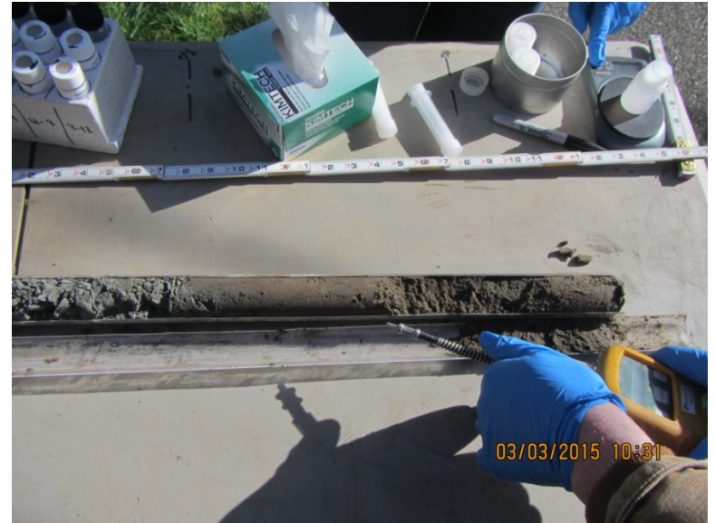
Photo 3. PID use for GP-11-A5 0-5ft bgs
