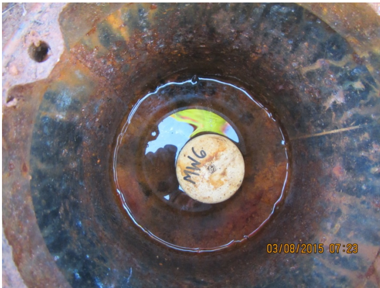
Photo 26. Monitoring well MW-6 with visible sheen in water within casing
