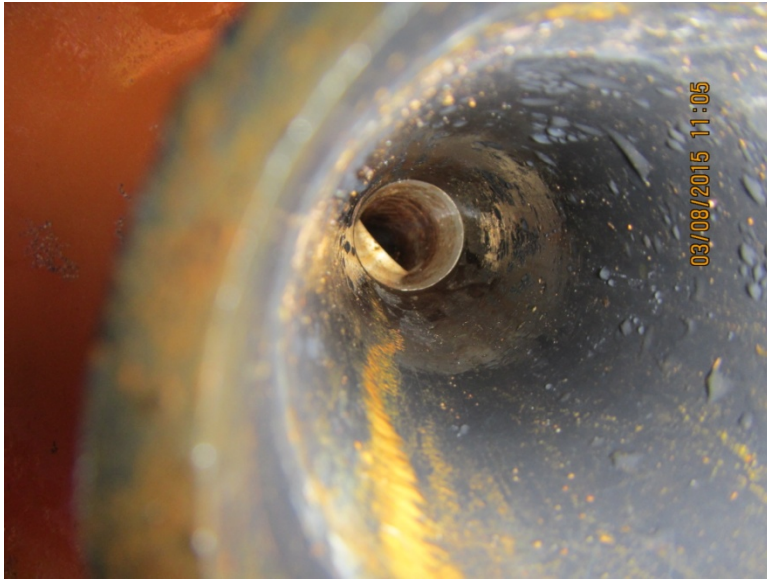
Photo 29. Suspected damage to riser in MW-5
