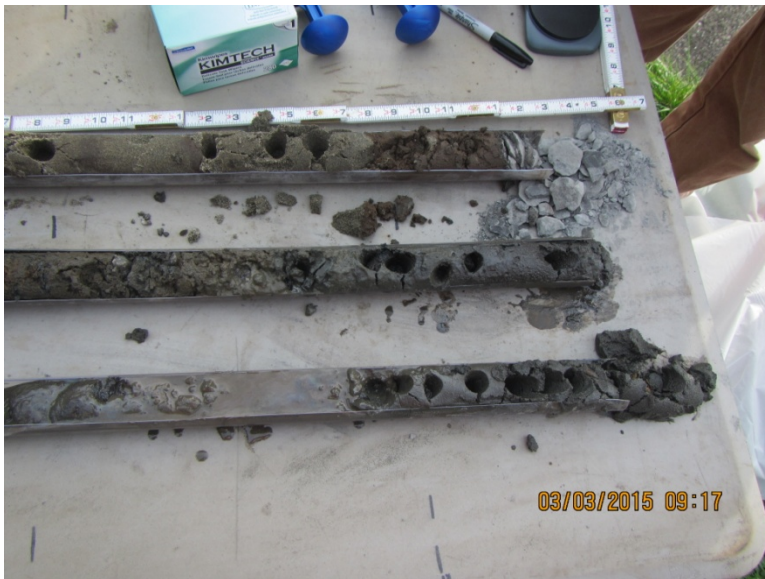
Photo 2. GP-11-A4 12.5-15.5 ft bgs with visible sheen
