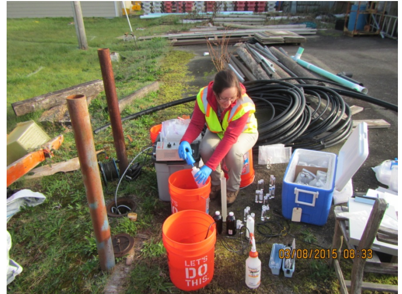
Photo 27. Sampling setup at MW-6
