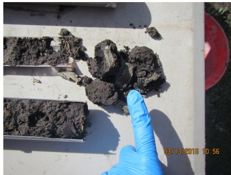
Photo 52. Wood chunks found in GP-11-E13 at approximately 4-5 ft bgs
