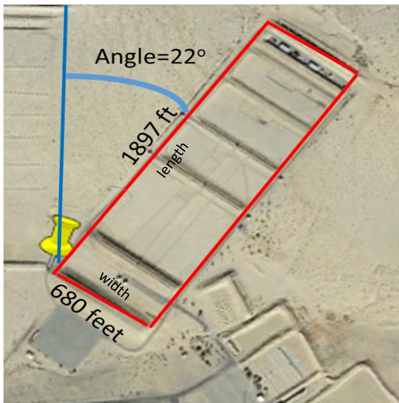
Figure 2-1. Example fugitive source characterization: NEI length = 1897 feet, width = 680 feet and angle = 22
