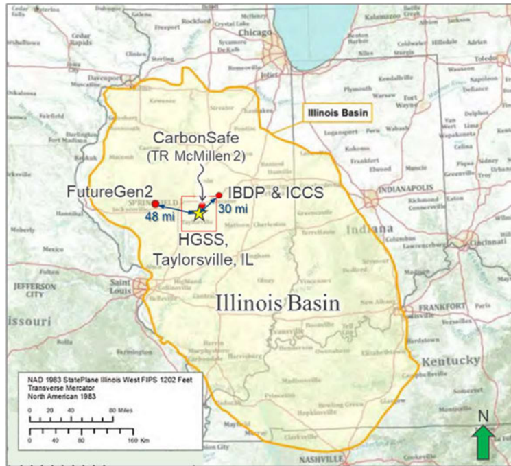
Figure 2-1. Illinois Basin map showing HGSS location and closest wells that penetrate the Mt. Simon. Red box represents Static Earth Model footprint.
