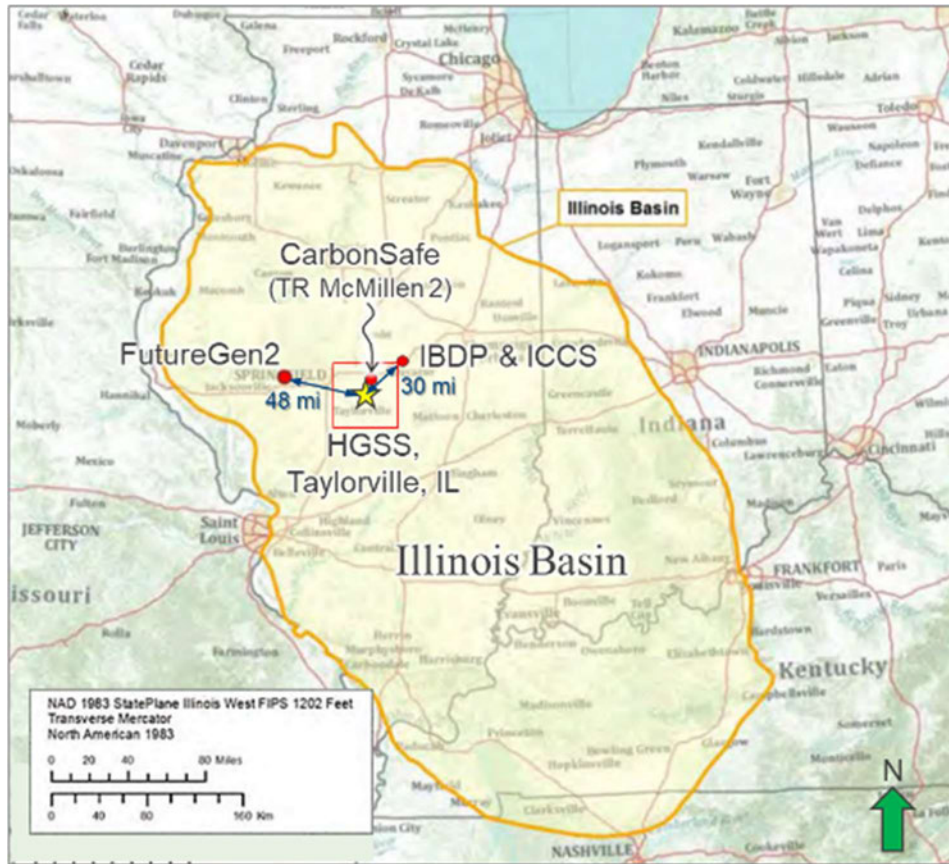
Figure 1-1. Illinois Basin map showing HGSS location and nearest wells that penetrate the Mt. Simon Sandstone. The well logs from the TR McMillen 2 well were used as an analog to model the caprock and reservoir for HGSS. The red box represents the 35x35 mile Static Earth Model footprint prepared for this permit.
