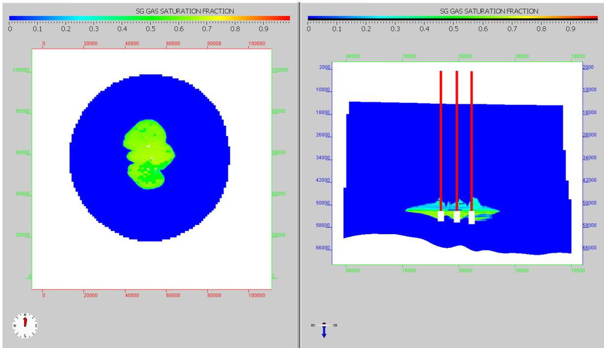
Figure 12. Plan and cross-sectional views of CO<sub>2</sub> saturation outlined by critical differential pressure front at the end of injection. Model coordinates (ft) are labeled on images. The plan view coordinates at the corners (in Decimal Degree NAD83) of: NE: -88.28294193, 40.63582357; SE: -88.28294299, 40.34439485; SW: -88.6648716, 40.34439586; NW: -88.66486794, 40.63582328.
