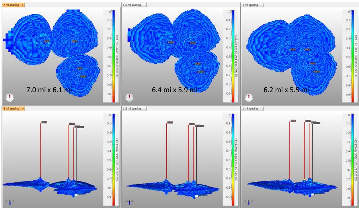
Figure 14. Plan and cross-sectional views of CO<sub>2</sub> plume at various well distances. (Distance between wells in upper left corner of each view.) Vertical exaggeration is 10x.
