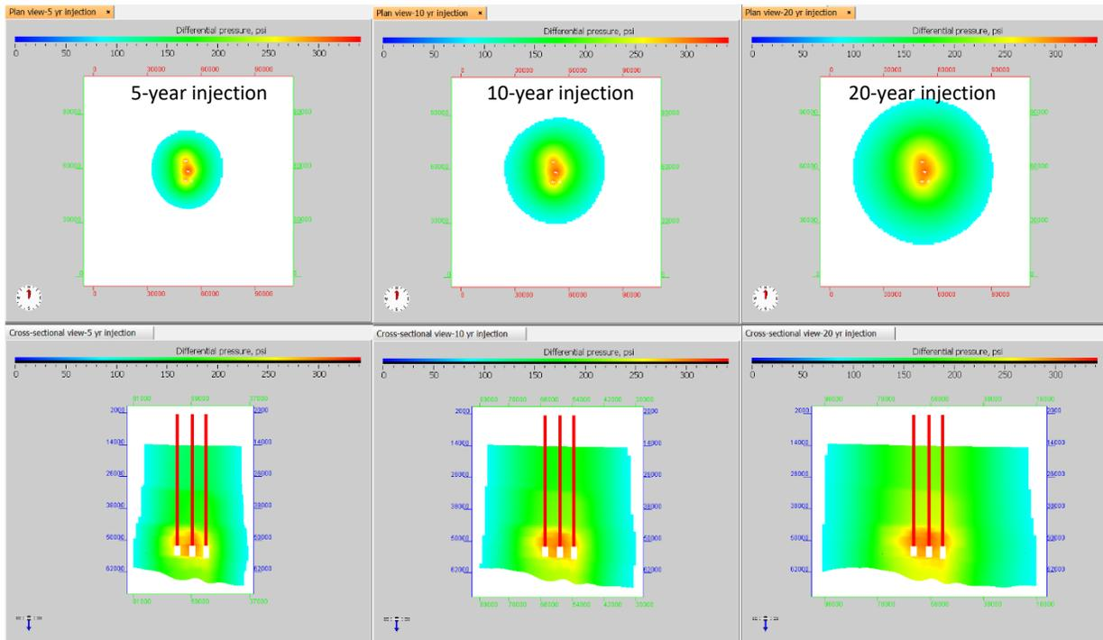
Figure 11. Plan and cross-sectional views of pressure front at 5, 10, and 20 years of injection (scale on each image is in feet).
