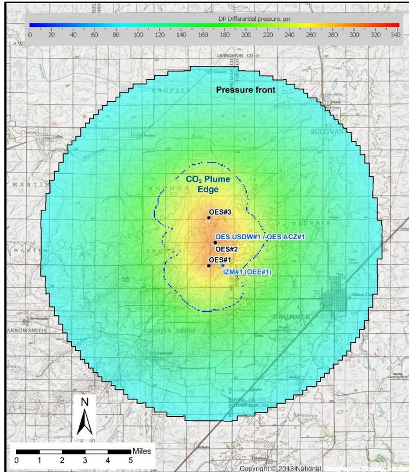
Figure 16. Predicted maximum AoR at 20 years of injection, shown overlain on a topographic map of the immediate area around the project wells. The map corner coordinates (Decimal Degree NAD83) are: NE: NE = -88.309199, 40.653973; SE = -88.309307, 40.352654; SW = -88.648213, 40.352227; NW = -88.649625, 40.653543.
