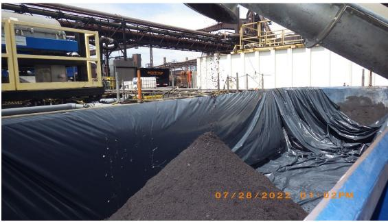
Description: Solids from the centrifuges are deposited into dumpsters for disposal. Location: Reclamation Services Building. Camera Direction: Northeast. Date/Time: July 28, 2022/1:02 P.M.
