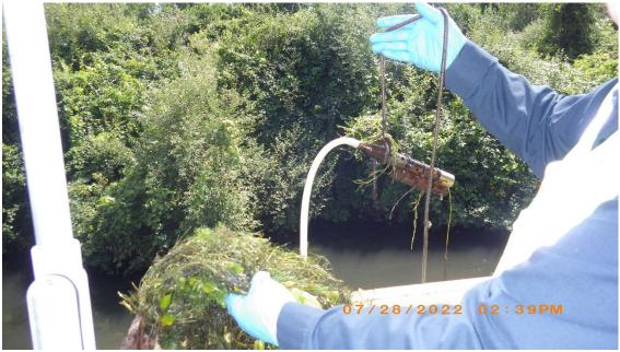
15: CHWW0071Description: Sample tube for Outfall 011 catches stream vegetation.Location: Outfall 011.Camera Direction: South.Date/Time: July 28, 2022/2:39 P.M.
