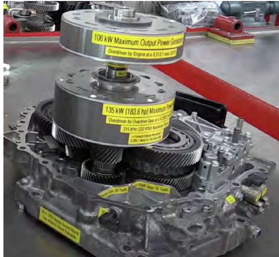
Figure 2-28: An example of a series/parallel hybrid drive system for a transverse/front-drive application with a portion of the outer casing and stators removed to show internal details. Adapted from a presentation by Prof. J.D. Kelly, Weber State University (Kelly 2020).
