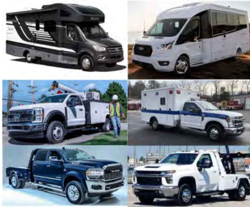
Figure 3-8: Examples of incomplete MDV chassis finished with customized bodies for specific applications.
