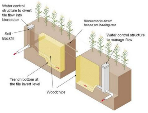
Figure 1. Bioreactor. (Source: Cohen 2016)
