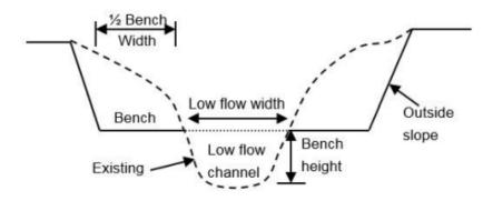
Figure 9. Illustration comparing a conventional ditch (*dotted line*) and a two-stage ditch (*solid line*). (*Source*: NRCS, Indiana 2018)
