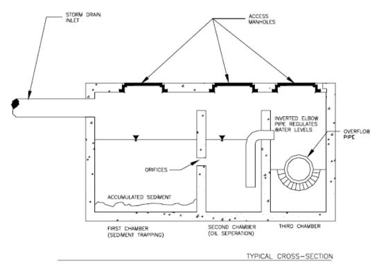
Figure 15. Oil/Grit Separator schematic. (Source: adapted from Schueler 1987, cited in MassHighway 2004)
