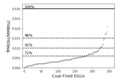
Figure 1—fPM rate distribution for affected coal-fired EGUs in the continental U.S. in reference to the three considered fPM limit (horizontal dashed lines): 1.5E-02 lb/MMBtu, 1.0E-02 lb/MMBtu, and 6.0E-03 lb/MMBtu. Percentages represent the amount of existing capacity achieving each of the limits. More information available in the Technical Memo supporting this action.
