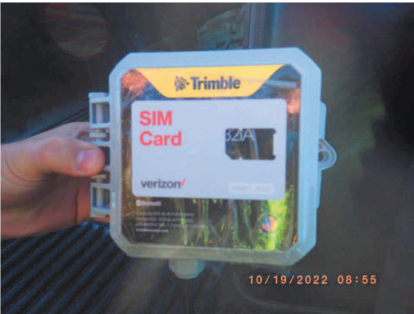
17: RIMG1617 Description: Pressure Monitoring Equipment
