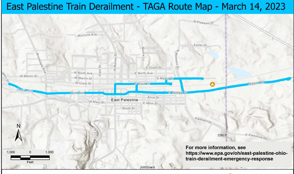
On March 14, 2023, EPA's Trace Atmospheric Gas Analyzer (TAGA) bus performed air monitoring around the East Palestine Derailment Location, monitoring for n-Butyl Acrylate.
