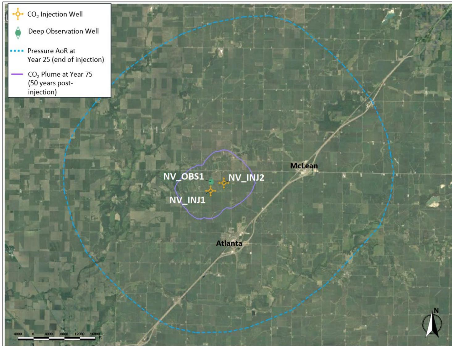
Figure 17: Predicted maximum extent of the project AoR, as predicted by the 137-psi delta pressure at the end of the operational phase of the project in Year 25 (end of injection). The outline of the CO<sub>2</sub> plume at 50 years post-injection (Year 75) is also shown. NV\_INJ1 and NV\_INJ2 are the injection wells, and NV\_OBS1 is the observation well.
