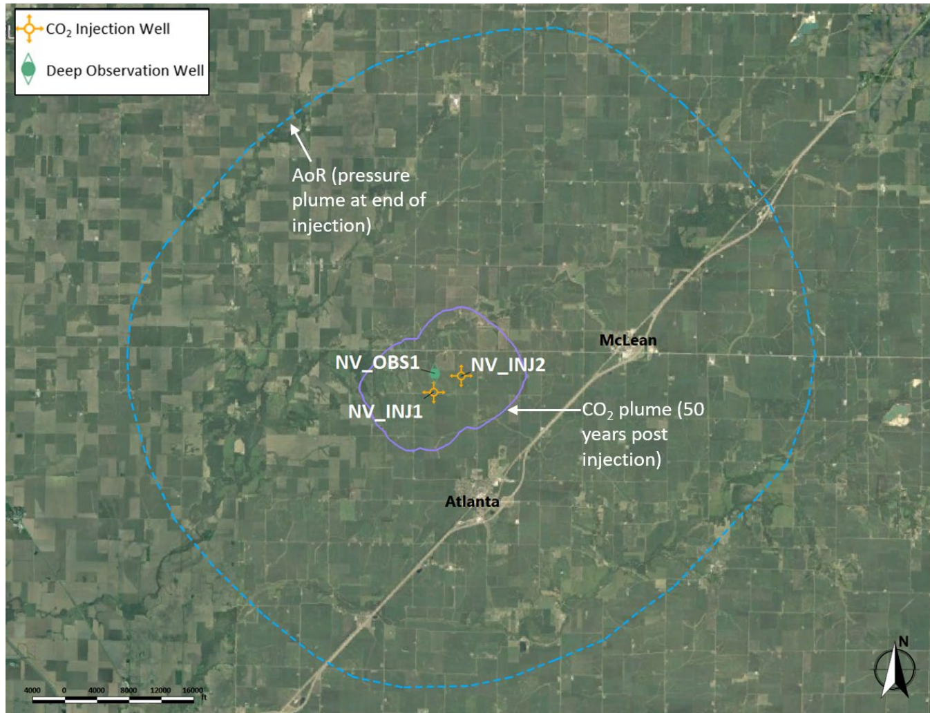
Figure 1: Map of the project AoR, as predicted by the 137-psi delta pressure at the end of the operational phase of the project. The outline of the CO 2 plume at 50 years post-injection is also shown. NV_INJ1 and NV_INJ2 are injection wells and NV_OBS is the deep observation well.
