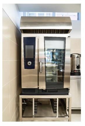
oven is in operation. In contrast, boilerless combination ovens have a self-contained water reservoir that is used to spray water directly on a heat source to create the steam for cooking. This eliminates the use of a separate, central boiler system and saves energy that would have been used to supply continuous steam. Boilerless combination ovens are typically drained and refilled each day and do not require a drain of condensate or the addition of cooling water.
