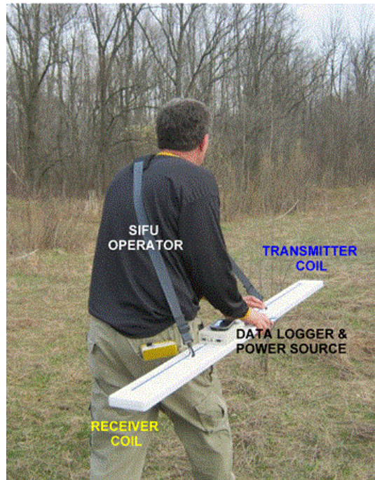
Figure 1: GEM-2 Electromagnetic Induction Survey in Progress
