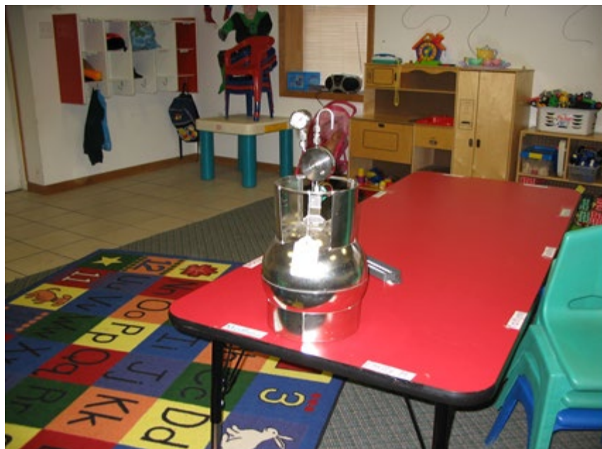
Example of a canister with a regulator attached and placed in the breathing zone.
