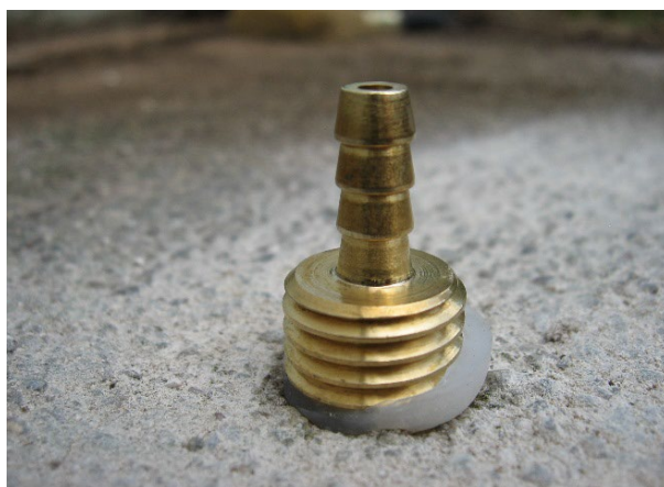
Figure 3: Vapor Pin™ installed and ready for sampling
