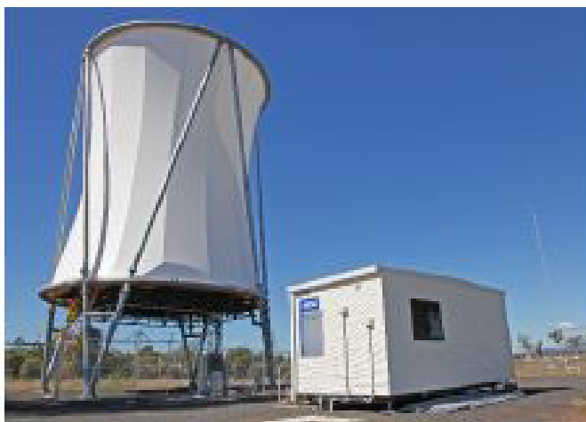
Figure 4-8. Demonstration Hybrid Cooling Unit (from Gwynn et al., undated).
