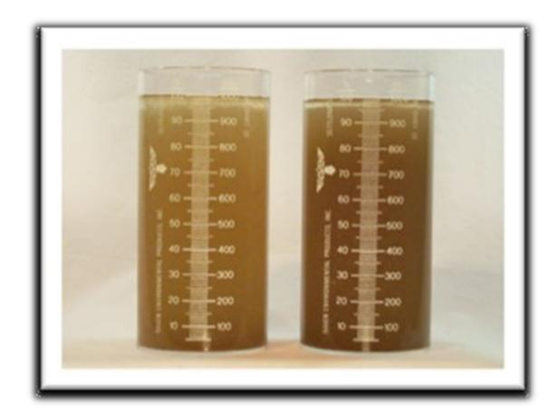
The Settleometer on the LEFT in each photo - the mixed liquor is diluted 50% with clarifier effluent The Settleometer on the RIGHT in each photo is 100% mixed liquor
