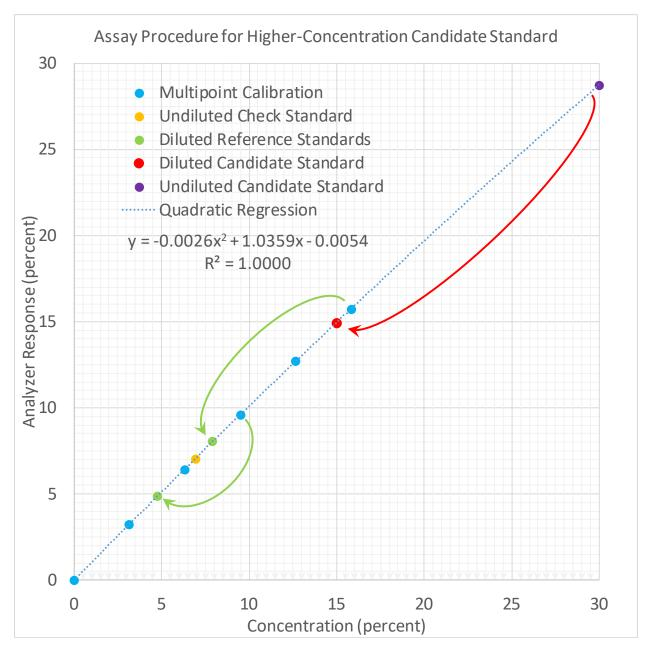
This proposed procedure failed to account for the fact that the physical and thermal characteristics of high-concentration  $CO_2$  gas mixtures vary significantly as the concentration varies significantly. This variation has significant effects on the k-factors for mass flow controllers and viscosity effects for gas dividers, which prevent mass flow controllers and gas dividers from diluting the gas mixtures accurately.
