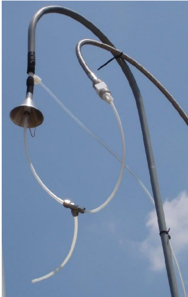
Figure 5-3. Hard Connection to Station Sampling Inlet
