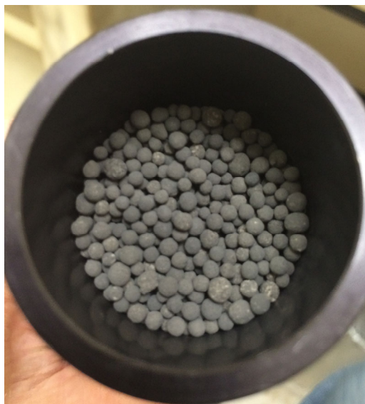
Figure A-3: Addition of Palladium Coated Pellets
