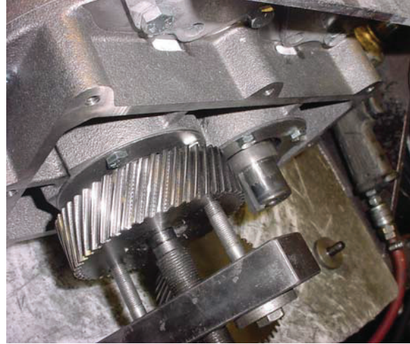
Figure 8-4 – Pulling Driven Gear with Bar Puller
