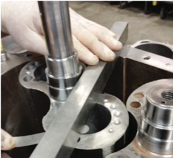
Figure 8-13 – Check Drive End Clearances
