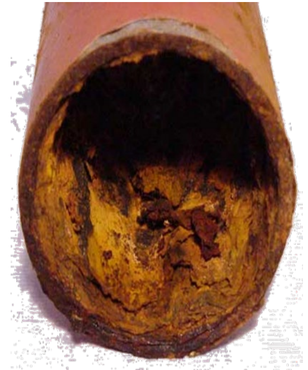
Rusted iron water pipe
