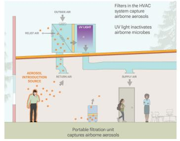
Figure 2: Sources of airborne aerosols and their infiltration
