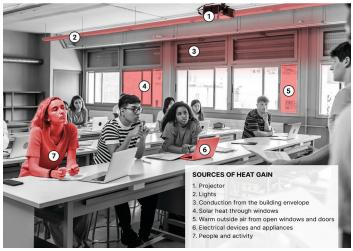
Figure 1: Sources of heat within a typical classroom
