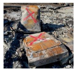
**Red paint** = Lithium battery power walls or photovoltaic equipment.
