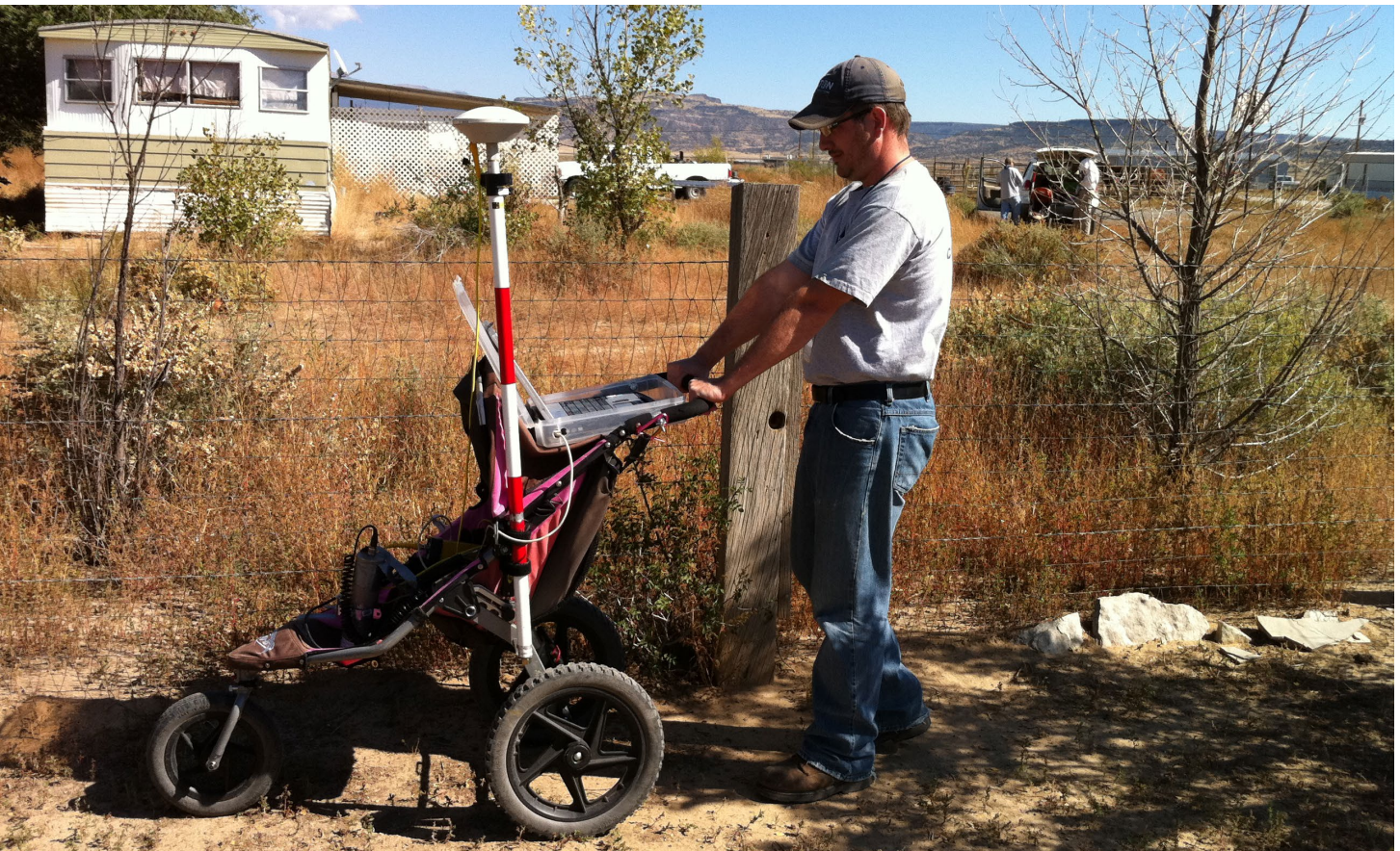
EPA Contractor conducting a residential gamma survey. The buggy contains GPS and measuring instruments.
