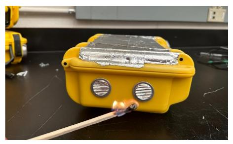
Sensor test using a lit match to check for PM, CO<sub>2</sub>, VOC sensor response
