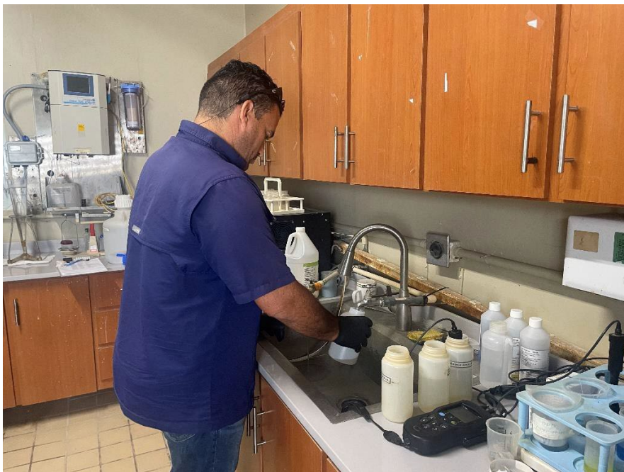
Photograph 10: View of START V team member collecting influent drinking water samples at the Guayama DW Treatment plant.
