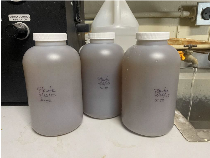
Photograph 11: View of influent drinking water samples collected from the Guayama DW Treatment Plant.
