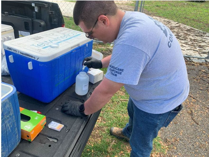
Photograph 5: View of a START V team member preserving a drinking water sample with nitric acid.
