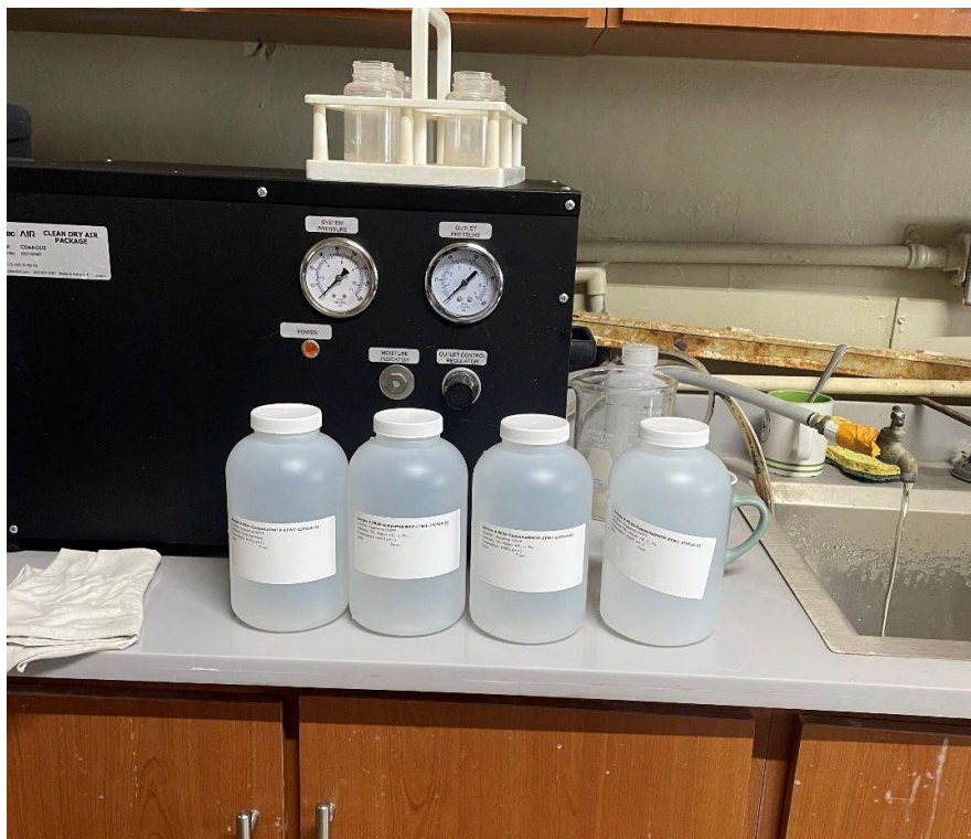
Photograph 2: View of effluent water samples collected at the Guayama DWTP, including field duplicate and additional sample volume designated as matrix spike/matrix spike duplicate (MS/MSD).
