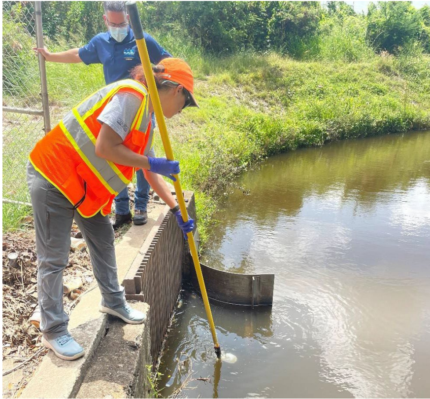
Photograph 9: View of START V collecting raw water samples. Samples were taken from the entrance of the irrigation channel to the Rexmanor Pump Station located at latitude 17.98077°, longitude -66.10087°.
