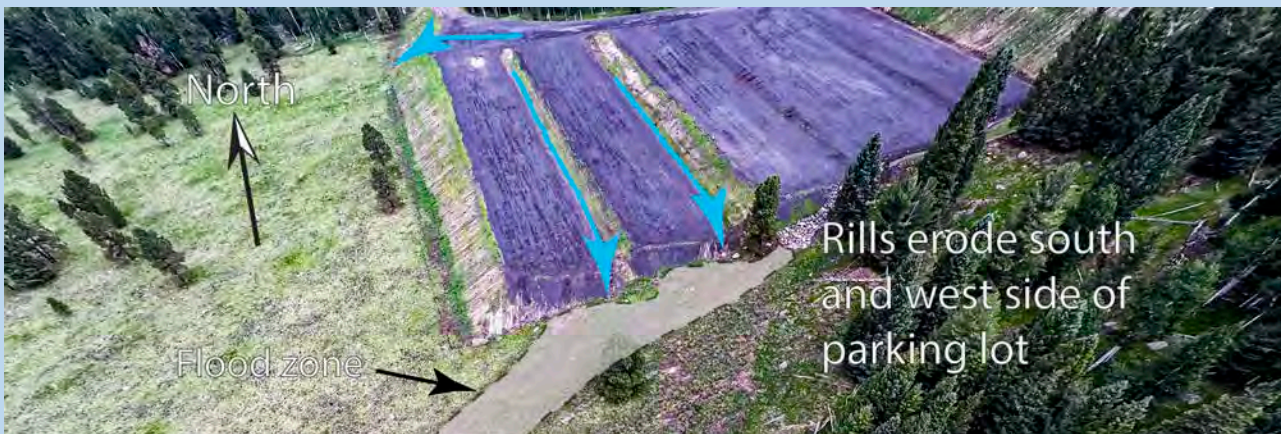
Left, rills were eroded into south and west-facing sides of parking lot during late July runoff. Right, rill of farthest west of two channels.
