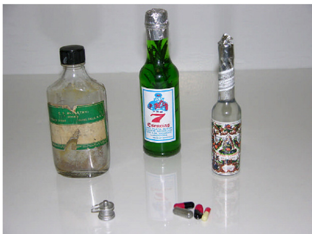
Fig. 1 – Foreground left: amalgam icon — Parad Shivling. This item weighed 10 g and emitted 0.3 \mu\text{g}/\text{h} \text{Hg}^0 vapor at 24 °C. Foreground right: gelatin capsules containing \text{Hg}^0 . The clear capsule contains 9 g \text{Hg}^0 and was purchased in the study area for $1.00. We purchased the colored capsules in the Dominican Republic at a similar cost. Rear left: bottle of elemental mercury. This bottle contains approximately 2 kg \text{Hg}^0 and was the source of spilled Hg in the reference community (C1). Rear center and right: Agua de Florida, and 7 Escencias. We purchased these items in the Dominican Republic also. The store clerk suggested we mix these items with mercury from the capsules and apply the mixture to floors in the home twice per week. These products typically contain water, alcohol, and essential oils. We do not believe they contain mercury though we did not analyze them.
