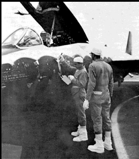
Figure 40. Final check after B-57 decontamination, Naval Air Station, Operation DOMINIC.
