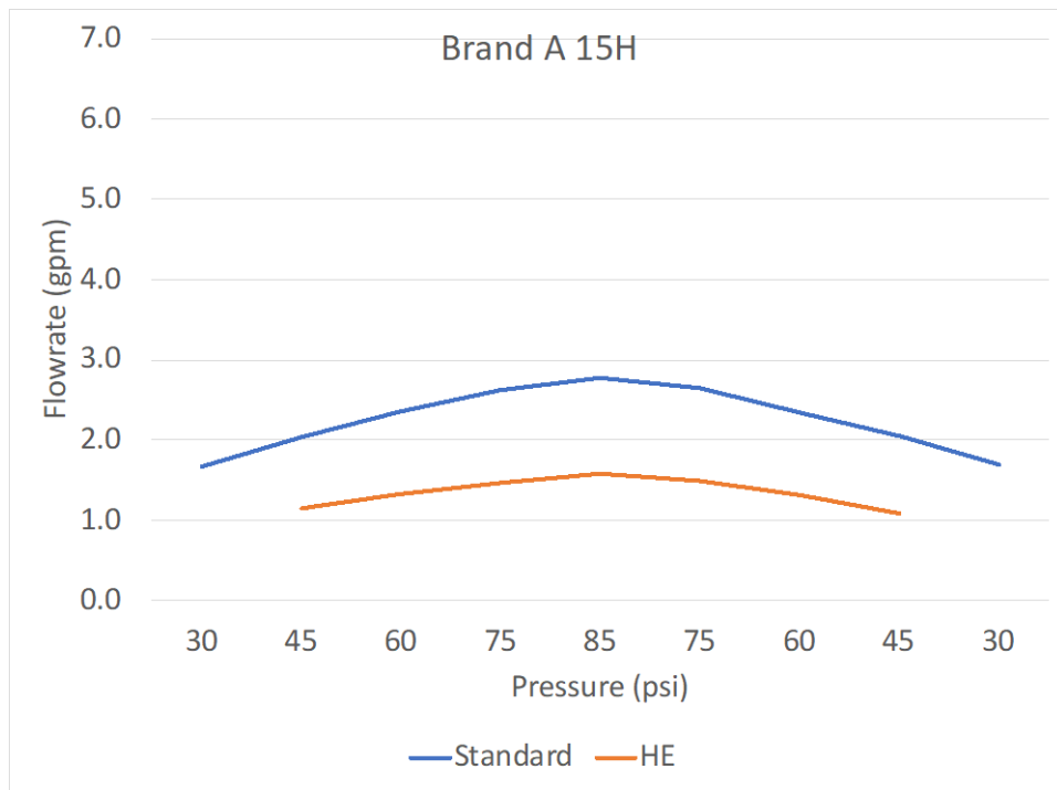
Figure 7. Flowrate curve from Brand A 15F and 15H standard nozzles and analogous radii HE nozzles
