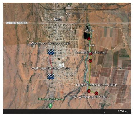
Figure 6. Alternative B – proposed West Creek debris removal location and existing effluent disposal pipeline
