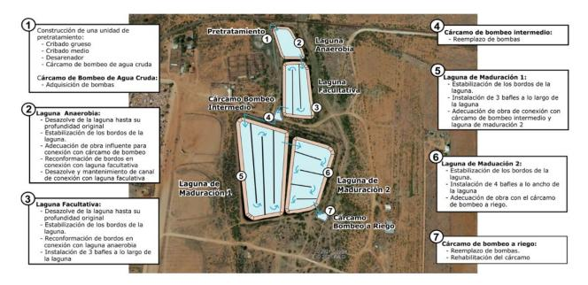
Figure 7. Alternative B – proposed lagoon rehabilitation actions
