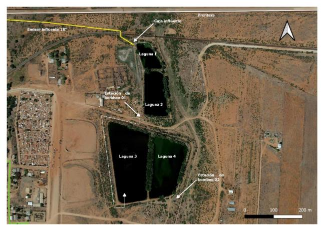
Figure 3. Alternative A – existing wastewater treatment system
