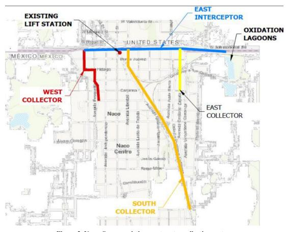
Figure 2. Naco, Sonora existing wastewater collection system
