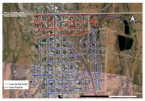
Figure 5. Alternative B – wastewater collection system replacements (indicated in red)
