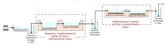
Figure 8. Alternative B – Proposed wastewater treatment flow diagram
