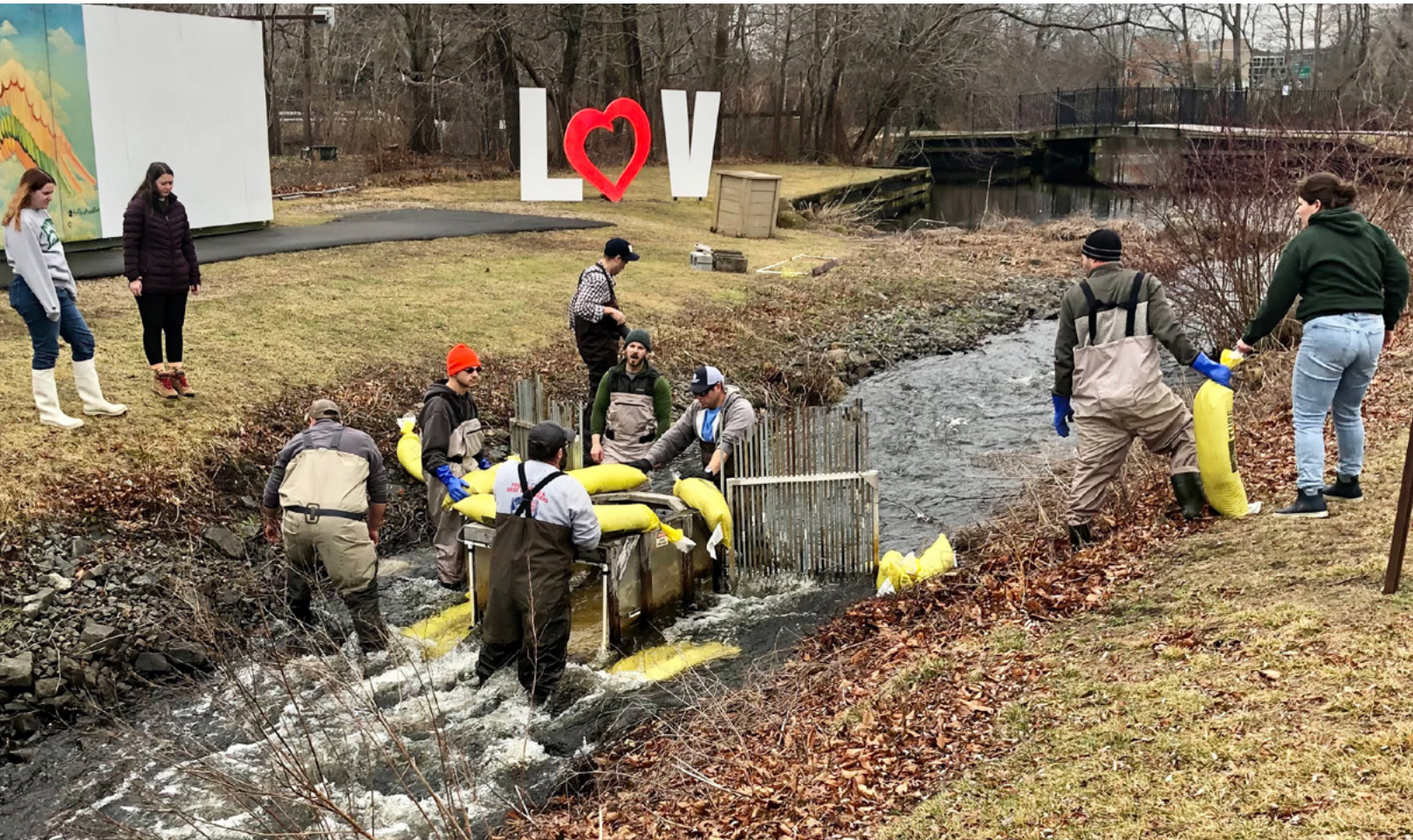
Volunteers from the Suffolk County Community College install a fish counter to monitor alewife and American eel on the Peconic River at Grangebél Park, Riverhead, New York. Photo by the Peconic Estuary Partnership
