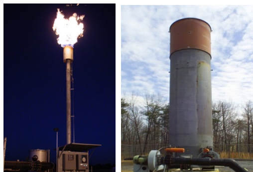
Figure 1-4. Open (left) and Enclosed (right) Flares
