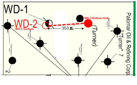
WD-1: Surface and bottom hole locations are 859' South and 2,152' East of the NW corner of Sec 23, T29S, R27E.
