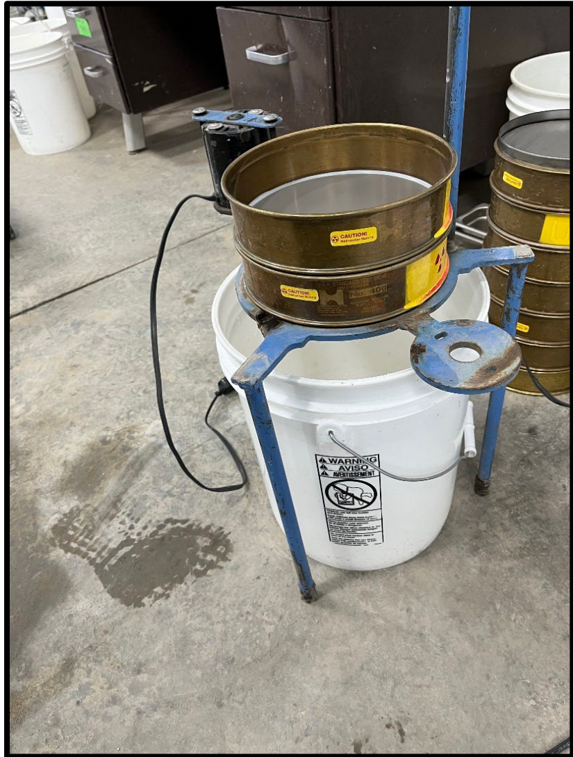
Figure 22. Vibratory Sieve Shaker Used for Wet Sieving Determination of Particle Size Distribution at the Disa Process Laboratory Post-Field Study
