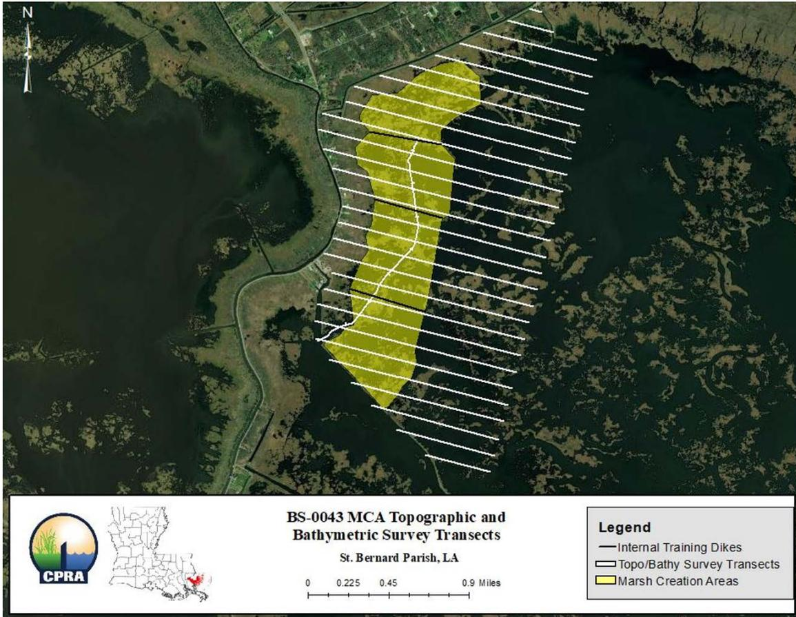
**Figure 12:** MCA Topographic & Bathymetric Survey Transects.
