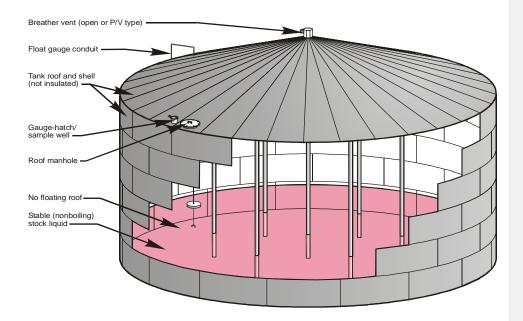
Figure 7.1-1. Typical fixed-roof tank.<sup>2020</sup>
