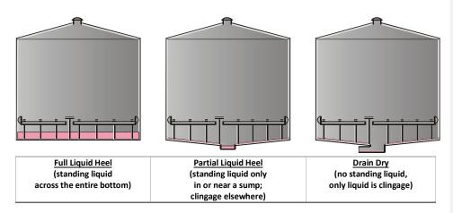
Figure 7.1-20. Bottom conditions for landing loss.<sup>2020</sup>
