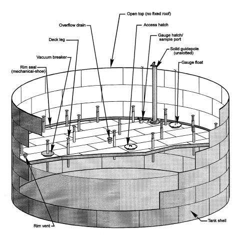
**Figure 7.1-3**. External floating roof tank (double deck).<sup>20</sup>
