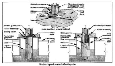
Figure 7.1-11. Slotted and unslotted guidepoles.<sup>20,20</sup>
