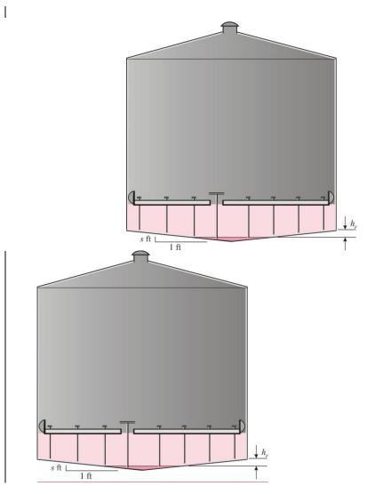
**Figure 7.1-24.** Depth of a partial heel in a cone down bottom. <sup>20</sup> This figure illustrates a variable used in Table 7.1-4.
