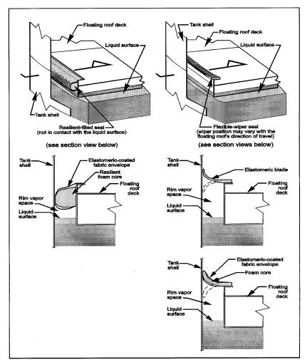
Figure 7.1-6. Vapor-mounted primary seals<sup>20</sup> seals<sup>20</sup>
