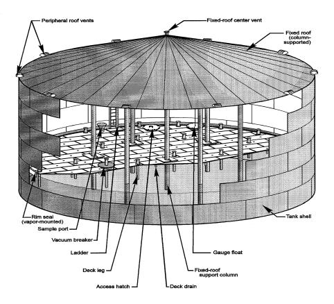
Figure 7.1-4. Internal floating roof tank.<sup>20</sup>
