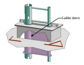
Figure 7.1-21. Ladder-slotted guidepole combination with ladder sleeve. <sup>20</sup>
