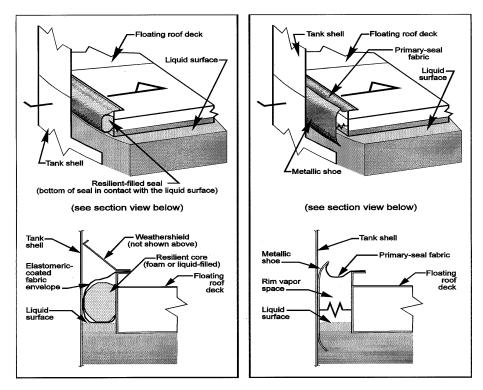
Figure 7.1-7. Liquid-mounted and mechanical shoe primary seals.  $\frac{29.20}{20}$
