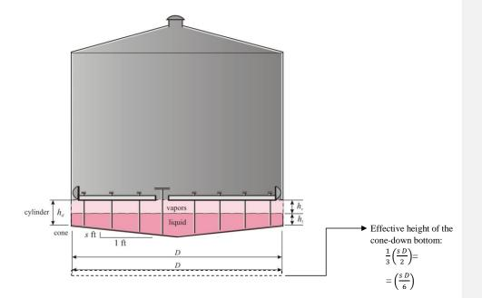
**Figure 7.1-23**. Height of the liquid heel and vapor space under a landed floating roof.<sup>20</sup> This figure illustrates variables used in Table 7.1-4.
