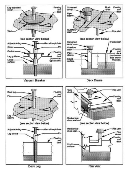
Figure 7.1-10. Deck fittings for floating roof tanks.<sup>20,20</sup>
