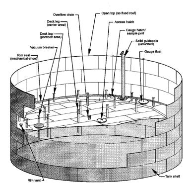
**Figure 7.1-2**. External floating roof tank (pontoon type).<sup>20</sup>
