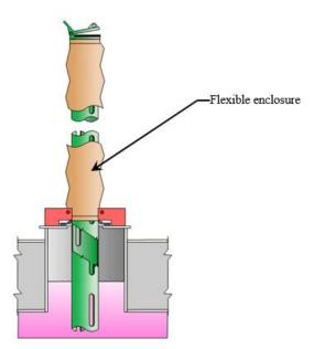
Figure 7.1-22. Slotted-guidepole with flexible enclosure.<sup>20</sup>
