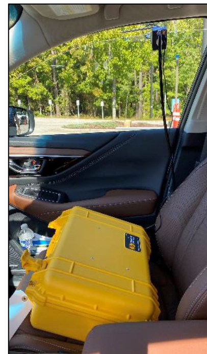
Vehicle add-on mobile monitoring system (VAMMS)
