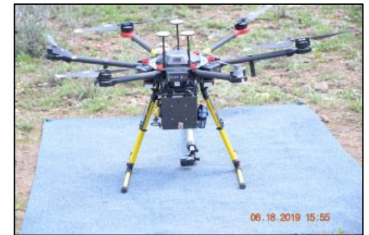
Kolibri air sampling system attached to a small unmanned aerial system
