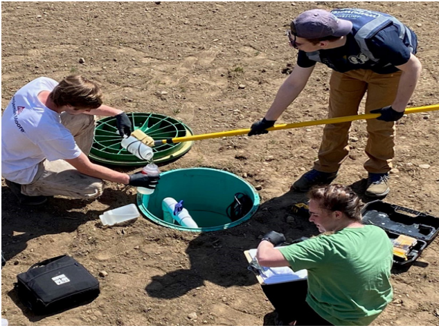
University of Rhode Island students and Town of Charlestown staff sampling a septic tank preceding an LSTA drainfield to determine nitrogen removal. Photo credit: Matthew Dowling
